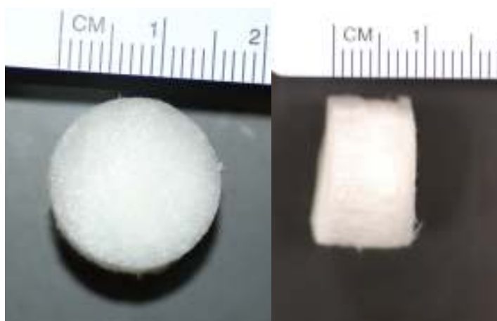
Figure 3-1. Optical Images of Lyophilized Collagen Scaffolds Prior to Hydration and Crosslinking.
